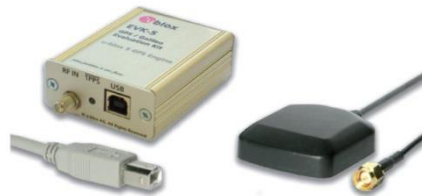
Figure 5: uBlox EVK-5T GPS Development Kit
